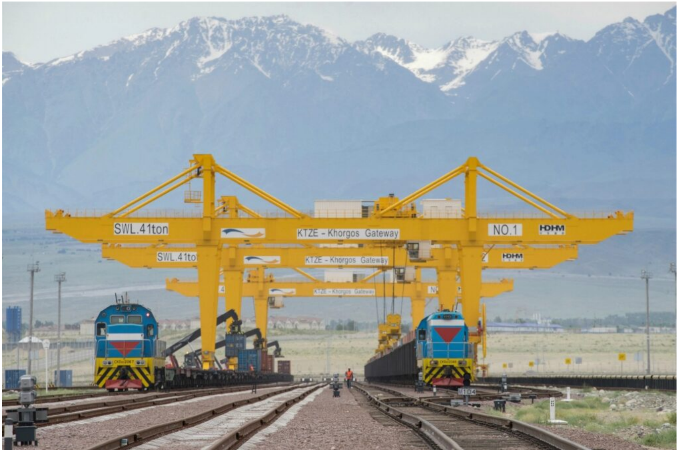
Trains of different gauges, from China and Kazakhstan, transferring loads at the Khorgos “dry port” (Image: Alamy)
